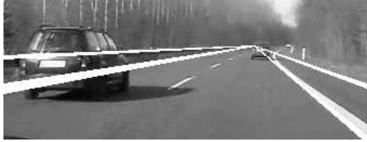
Fig. 7. Lane Border Detection
