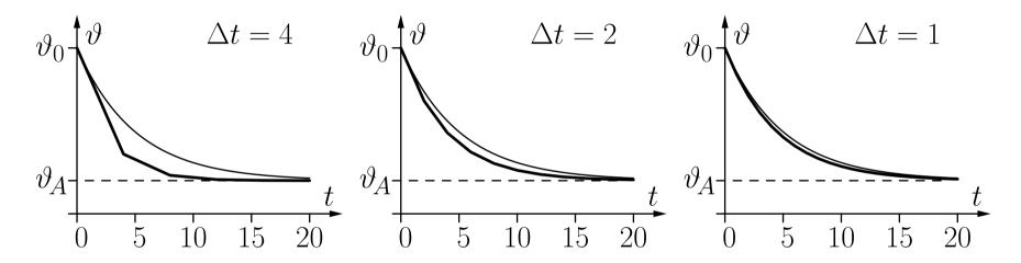
The thin curve is the exact analytical solution.
