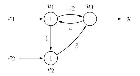
$$f_{\text{net}}^{(u)}(\vec{w}_u, \vec{n}_u) = \sum_{v \in \text{pred}(u)} w_{uv} \text{in}_{uv} = \sum_{v \in \text{pred}(u)} w_{uv} \text{out}_v$$
