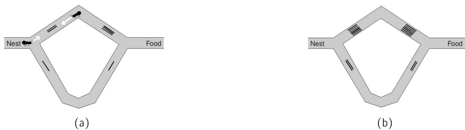
Figure 2.5: (a) Via the ants' biased choice the amount of pheromone on the shortest paths is rising steadily. (b) After a certain time most ants take the shortest paths; even though the longer branch is also taken by a small number of ants.
