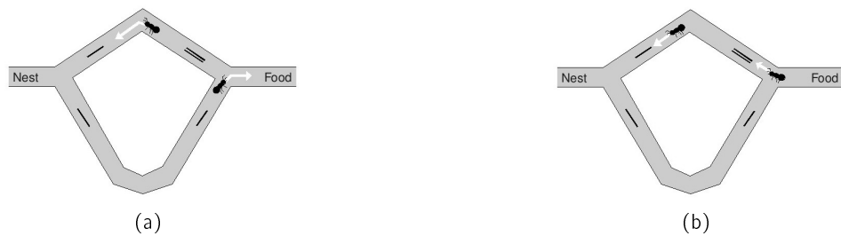
Figure 2.4: (a) Finally the second ant arrives at the food source and (b) makes its decision for the return paths biased towards the pheromone: one pheromone unit on the longer branch and two units on the shorter branch. So it is likely that the second ant takes the shortest path, as well.
