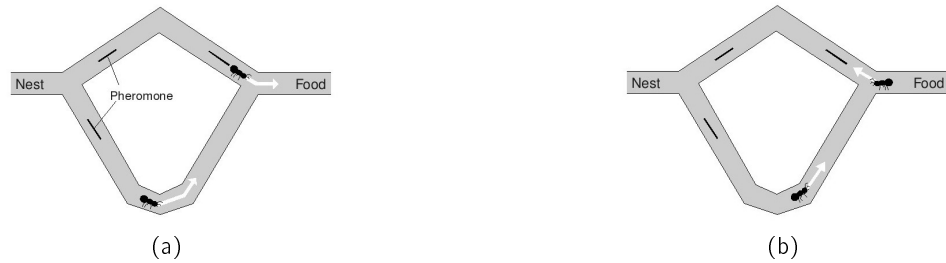
Figure 2.3: (a) By using a trail, ants deposit pheromone on it. (b) The ant that has taken the shorter path arrives earlier at the food source. On its way back to the nest, it has to make a choice which is now biased towards the amount of pheromone on the branches. Very likely the ant returns via the same branch again, as there is already some pheromone on it.
