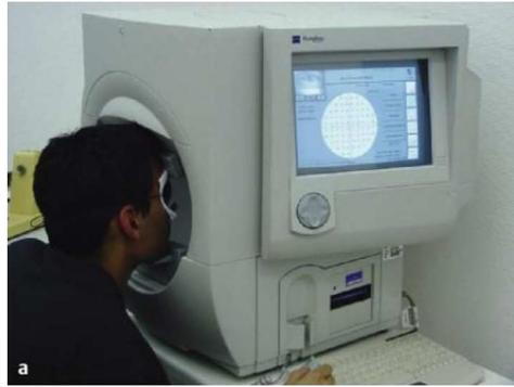
Figure 2.3: Humphrey Field Analyzer, source: [27, p. 395]
