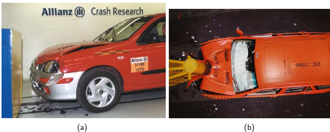
Figure 1.5: AZT (a) and frontal pole crash tests (b). The former type of crash is performed at 14 up to 16 km/h. Neither airbag, nor belt tensioner shall fire at these velocities. A frontal pole crash test shall reveal insights into frontal crashes with trees. (Both pictures are taken from [16])
