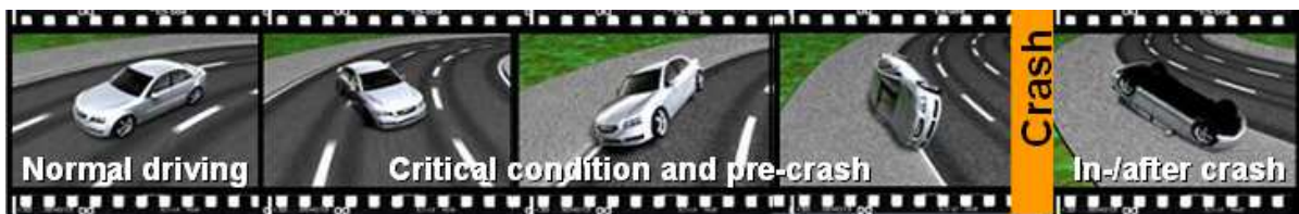
Figure 1.2: Phases of a crash [4]. In normal, critical or pre-crash situations, active safety systems may be used by the driver. On the other hand, passive safety systems are triggered automatically whilst in- and post-crash situations, respectively.
