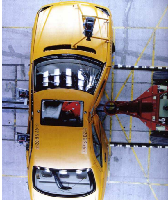
Figure 1.6: Lateral pole impact test [16] to gain information about real-world lateral tree crashes.
